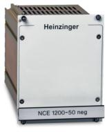
The Heinzinger NCE high voltage cassettes provide high voltage up to 30,000 Volts as a primary switched mode power supply, depending on the type and design, in a current range between 1 and 600 mA.
