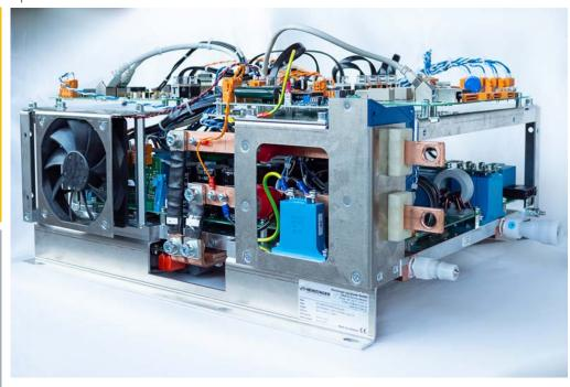
Ethernet Interface and watercooling are standard as well as 19" housing, where the components including infrastructure are installed.
